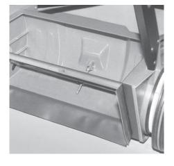
Remove three ea. Phillips screws, turn broom roller 180°, remove Phillips screws from second half. Pull the drive pin out of the broom shaft.
